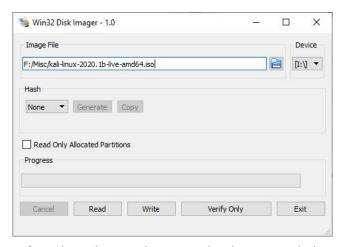
Ensure the writeto 'Device' is selected correctly. It must be the USB stick that you intend to burn the iso to, so check carefully that it is. If you accidently write to your hard drive, you will damage the operating system and all files, so be careful.
