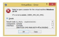
This related to 3 BIOS settings that needed to be switched on to allow the VirtualBox to utilise the computer's CPU. VTx and VTd needed to be selected (under Advanced) and this then allowed TXT to be selected which was under the Security tab. If you have an error, it may be different, and you will need to read the details and see what needs configuring. When I changed the BIOS settings and rebooted, Kali then ran in VirtualBox without any issues.
